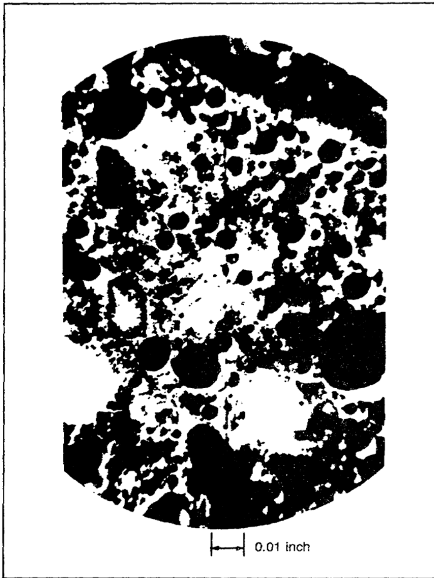
Figure 1-7. Polished section of air-entrained concrete magnified many times.
